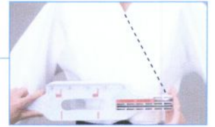
To check the width of the overlap points (more than 20cm)
